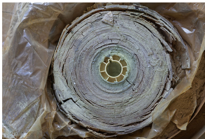
Film in advanced state of decay due to vinegar syndrome.
