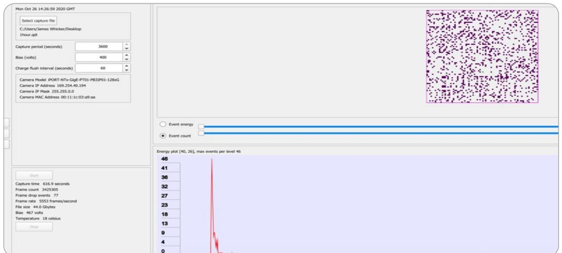
Figure 4: Example of data playback and energy spectra viewing within Quantum Detector's Helvellyn software. The user is able to select individual pixels and view the cumulative energy spectra at any point throughout the image acquisition.
