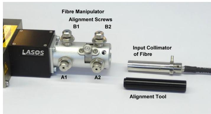
Fig. 38: Front end of the BDL-SMN laser. Beam profile corrector, fibre manipulator with alignment screws, input adapter of the single-mode fibre, and alignment tool.
