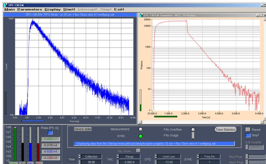
Fig. 33: Result obtained in the setup shown above. Fluorescence decay curve shown left, phosphorescence decay curve right. Both curves are recorded simultaneously.
