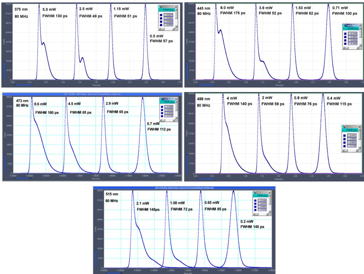
Fig. 23: Optical pulse shape for different laser power. Wavelength versions 375 nm, 445 nm, 473 nm, 488 nm, and 515 nm. Recorded with SPC-150N TCSPC module and id 100-20 detector. FWHM values corrected for 30 ps instrument response width.
