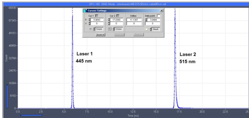
Fig. 30: Pulse-interleaved operation. 445 nm and 515 nm laser, Laser Sync cable 80 cm, repetition rate 50 MHz. The delay between the 445 nm and 515 nm pulse is 11.13 ns.
