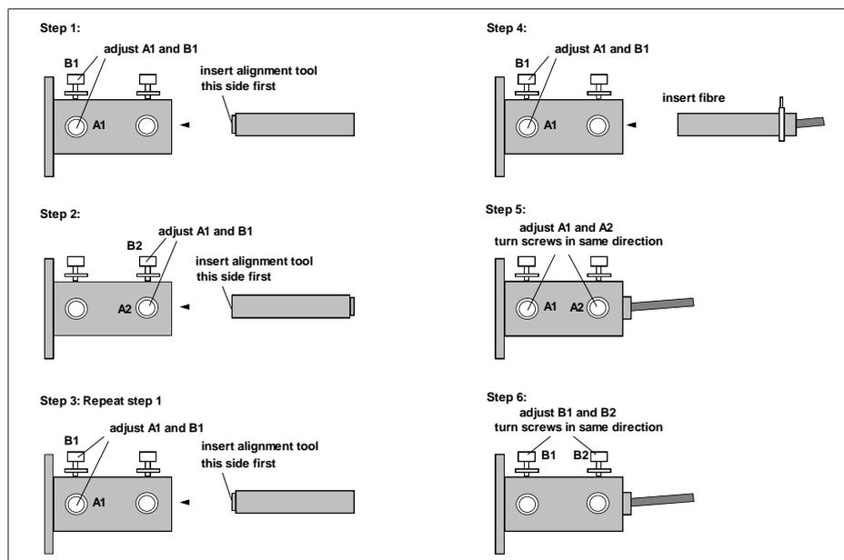
Fig. 39: Steps of the alignment procedure
