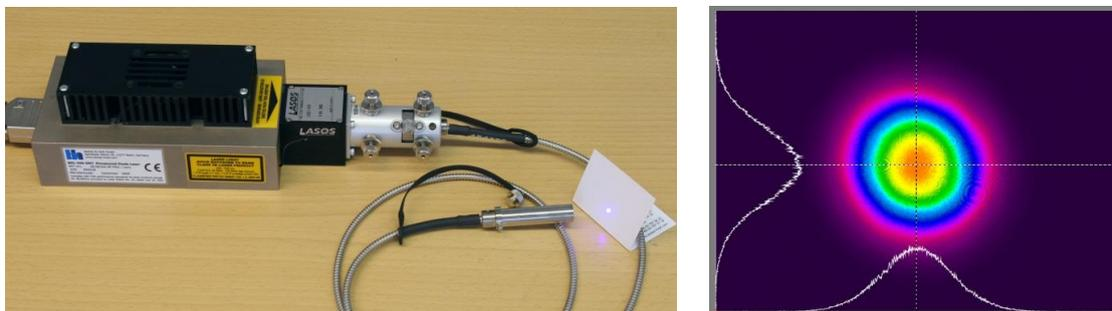
Fig. 20: Left: Collimated output from single-mode fibre. Right: Beam profile at the collimator output
