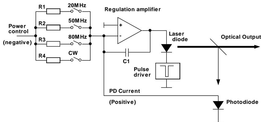
Fig. 24: Principle of power regulation loop
