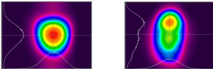
Fig. 19: Beam profiles in the CW mode. Left BDL-SMN 785 nm, Right: BDL-SMN 515 nm.
