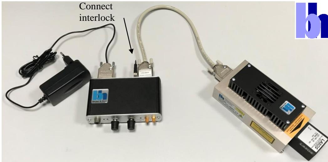
Fig. 1: BDL-SMN laser. Left: Wall mounted power supply. Middle: Switch box with safety key, frequency switch for CW and pulsed operation, power control and SMA connectors for external control. Right: Laser module containing the complete driving and control electronics.
