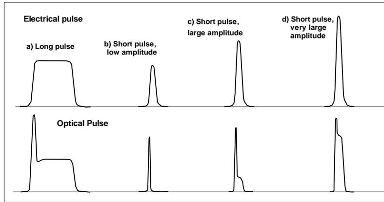
Fig. 22: Dependence of optical pulse on driving conditions of laser diode
