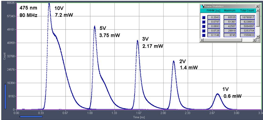
Fig. 6: Optical pulse shape and amplitude for different voltage of Power control signal. BDL-SMN 473 nm, 80 MHz. Power refers to free-beam output. Pulses recorded with SPC-150N TCSPC module and id100-20 SPAD detector.
