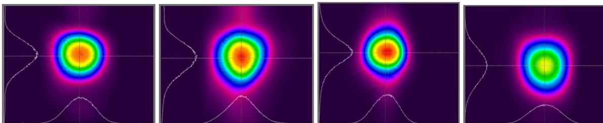
Fig. 18: Beam profile in 1m distance from the BDL-SMN laser, picosecond mode. Left to right: 405 nm, 473 nm, 515 nm, 785 nm version
