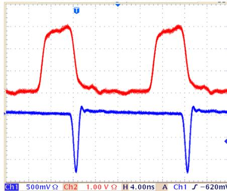
Fig. 13: Upper trace: Synchronisation signal to a second a second BDL-SMN laser, 1 V/div. Lower Trace: Sync signal to SPC modules, 500 mV/div. Time scale 4 ns/div. Repetition rate 50 MHz.
