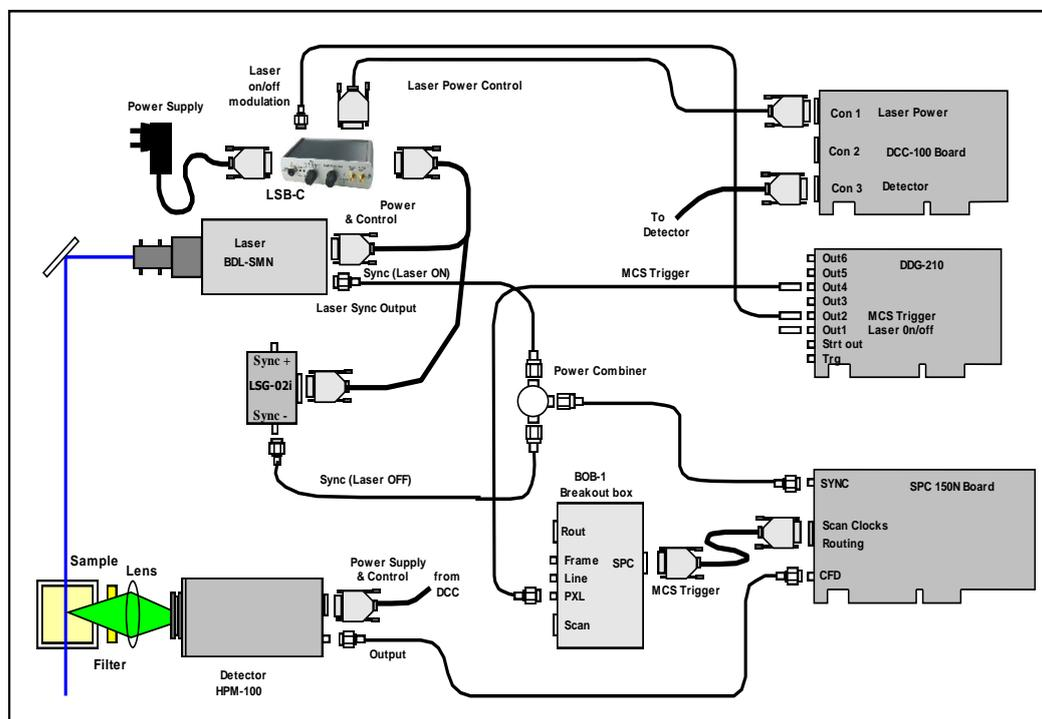
Fig. 32: Combined fluorescence / phosphorescence lifetime experiment
