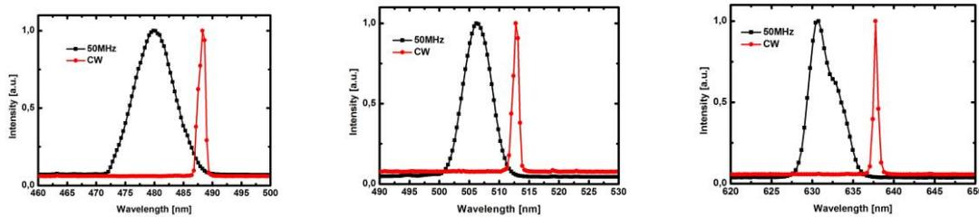
Fig. 21: Emission spectra for BDL-SMN lasers of different wavelength. Left to right: 488 nm, 515 , 640 nm. Please note different wavelength scales.
