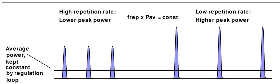
Fig. 25: The regulation loop keeps the average optical power constant. That means the peak power increases with decreasing repetition rate. The effect becomes apparent only with an external clock. For internal clock it is compensated by different resistors, R1 through R4, in the reference signal path.
