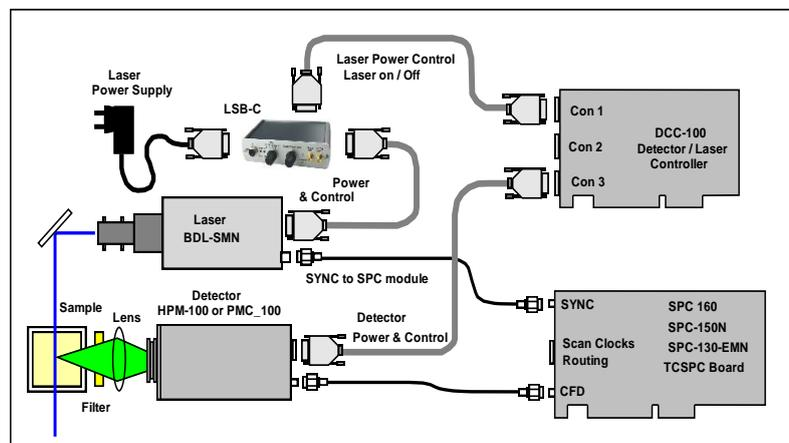
Fig. 28: Simple fluorescence-lifetime experiment
