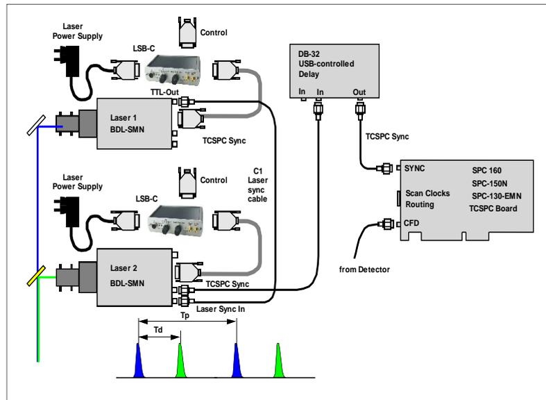
Fig. 29: System connections for pulse-interleaved operation of two lasers. Control connections to lasers not shown.
