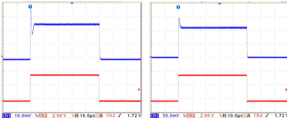
Fig. 9: Reaction of the optical power to the ON/OFF signal, picosecond operation, 50 MHz. Left: 10 % laser power. Right: 50 % laser power. Red curve: ON/OFF signal. Blue curve: Optical power. Time scale 10  $\mu$ s per division.
