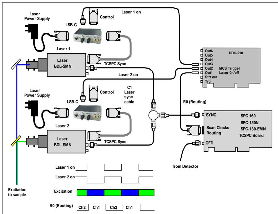
Fig. 31: Laser multiplexing. The lasers are switched ON/OFF alternatingly, the photons excited by each laser are stored in separate TCSPC memory channels
