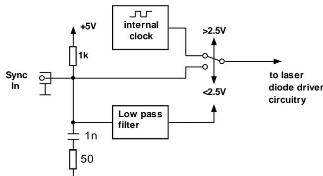
Fig. 14: Principle of switching between the internal clock generator and an external clock source
