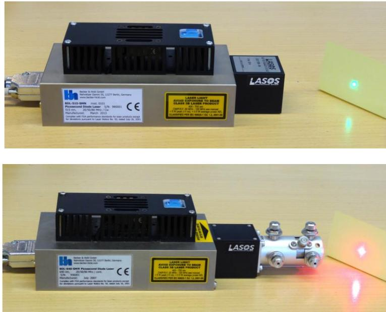
Fig. 17: Free-beam operation of the BDL-SMN laser
