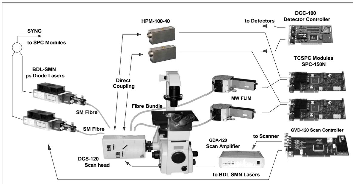
Fig. 34: Architecture of the DCS-120 confocal FLIM systems. Two BDL-SMN lasers are used for excitation. An example of a wavelength-multiplexed recording with two lasers is shown in Fig. 35.
