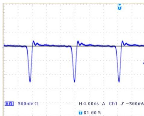
Fig. 12: Synchronisation signal to TCSPC modules. Repetition rate 50 MHz.
