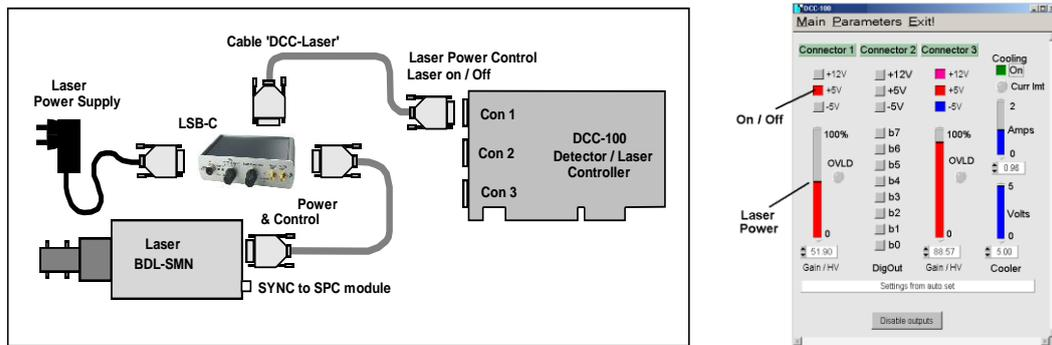
Fig. 27: Controlling the BDL-SMN from a DCC-100 Detector / Laser Controller card
