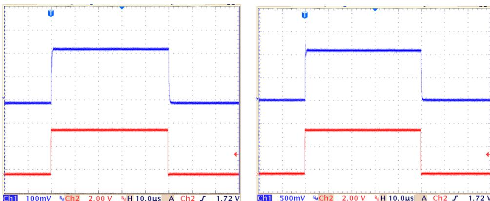
Fig. 10: Reaction of the optical power to the ON/OFF signal, CW operation. Left: 10 % laser power. Right: 50 % laser power. Red curve: ON/OFF signal. Blue curve: Optical power. Time scale 10  $\mu$ s per division.
