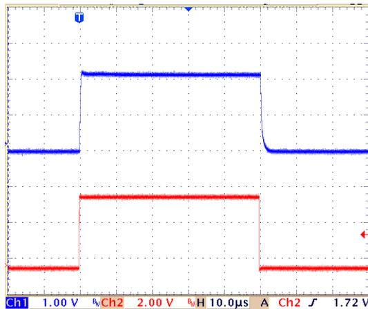
Fig. 8: Dynamic response of the output power to the power control signal CW mode. Control signal switches from 0 to +9 V. Time scale 10µs per division. Red: Control signal. Blue: Optical power.
