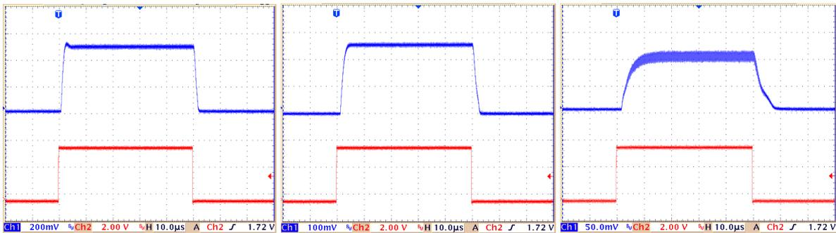
Fig. 7: Dynamic response of the output power to the power control signal. Control signal switches from 0 to +9V. Picosecond mode, 445 nm laser. Time scale 10µs per division. Red: Power control signal. Blue: Optical power. Left to right: Repetition rate 80 MHz, 50 MHz, 20 MHz. The noise in the 20 MHz curve is due to the pulsing of the laser.
