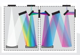
In **subtractive mode** the first and second stages work as a tuneable bandpass filter to allow only the desired portion of spectrum to pass through.
