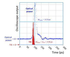
Optical pulse profile and timing interval error (TIE) from a 1550nm ID 3000 laser. Pulse width  $\Delta \tau_{pulse}$  is calculated as the FWHM of the optical pulse profile. Timing jitter  $\Delta \tau_{jitter}$  is calculated as the standard deviation of fluctuations in the detected optical pulse arrival time (the TIE), at 50% amplitude of the pulse's leading edge.
