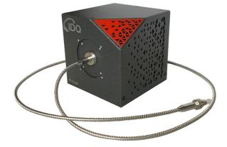
The detector offers a gate input designed to avoid saturation or undesired detections and can also be operated in Free-Running mode. The cooled InGaAs/InP avalanche photodiode and associated electronics have been specially designed to achieve low dark count and afterpulsing rates for fast gated operations.
