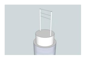
aluminium end cap. The end cap is machined to  $100~\mu m$  in the active area of the beam to minimise neutron scattering.
