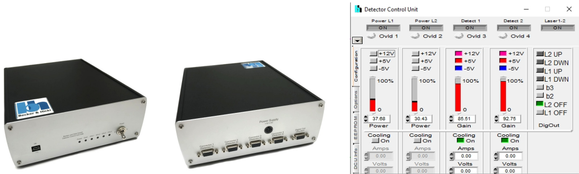
Fig. 4: Left and middle: DCU-400 detector/laser controller. Right: DCU software panel for control of two lasers and two detectors.
