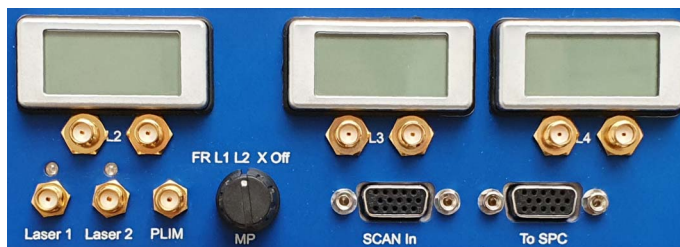
Fig. 7: Connection of the Scan clock signals through the MPM module. 'SCAN In' is the input from the scan controller, 'To SPC' is the output to the TCSPC module(s)
