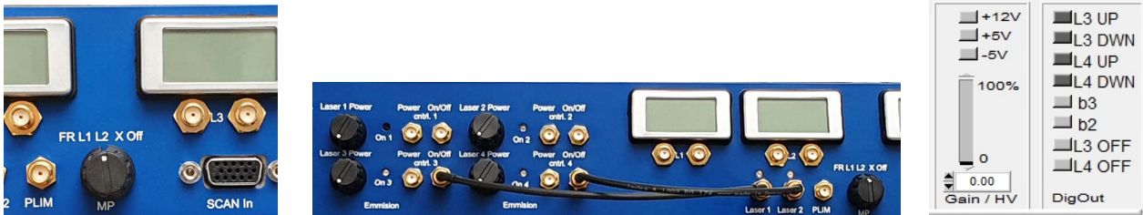
Fig. 6: Left: MPM mode switch. Middle: Cables from MPM to Laser ON inputs, lasers 3 and 4 are multiplexed by MPM outputs 1 and 2. Right: DCU panel with lasers 1 and 2 turned on
