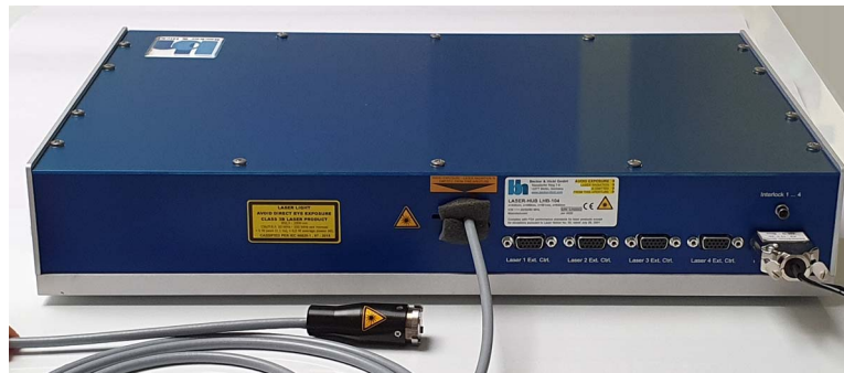
Fig. 11: LHB-104 with laser safety labels
