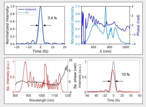
Left: Retrieved temporal profile and ideal Fourier transform limited shape (FTL). Right: Fiber output spectrum supporting 2.9 fs
