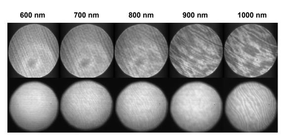
Data taken with white light source through a monochromator comparing etaloning performance of eXcelon vs. back-illuminated CCDs.
