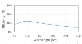
Grating efficiency into first order of diffraction. Total system efficiency  $\sim\!20x$  higher than conventional spectrometers due to proprietary no-slit technology
