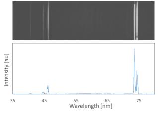
Sample spectrum from photoionized plasma of neon gas, produced by nanosecond midinfrared pulses and filtered by a 750um-thick aluminum foil
