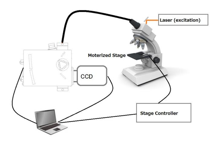
Instruments: Spectrograph, PIXIS, motorized stage
