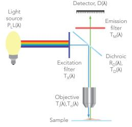
SearchLight Calculator takes into account all the spectral components of a typical epifluorescence microscope configuration. See Spectral Modeling in Fluorescence Microscopy, white paper for additional details.
