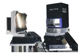
View of crystal and detector setup inside hiXAS. The HAPG crystal is specifically optimized to the target application. Extremely high resolving power and high efficiency are obtained simultaneously. The hybrid detector with large sensor area enables in-situ measurements.
